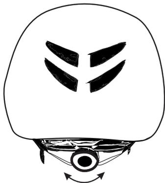
1. The headband adjuster wheel is turned to fit the headband to the head. See diagram 2.
