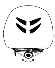
1. The headband adjuster wheel is turned to fit the headband to the head. See diagram 2.
